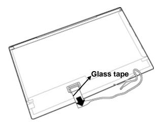
Figure 4-48 Removing the LCD cable
